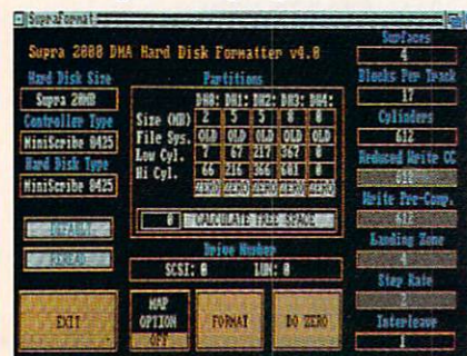
Above: the SupraDrive interface card. The empty sockets will be used for hard drive autoboot ROMs under Workbench 1.3 or later releases. Left: the Supra-Format working screen shows four partitions on this 20 meg hard drive.
